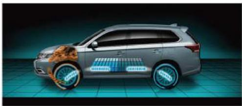
**Parallel Hybrid Mode: Engine power + motor assistance**
